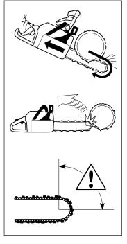
Cutting with the bottom edge of the bar, i.e. from the top of the object downwards, is known as cutting on the pull stroke.
